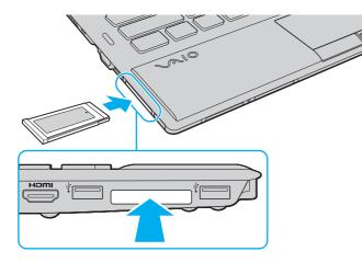
$\swarrow$  If the module does not go into the slot easily, remove it gently and verify you are inserting it in the proper direction.
